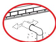
Make sure that the smoke outlet is as direct as possible to avoid incorrect air circulation.
