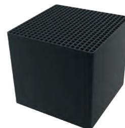
The dissociated recirculation - Box R allocates 9 to 10 Helsa charcoal cubes creating a system that enables up to 4000 parallel flow channels, capturing grease and odours very effectively. By separating the air in multitude of channels, this system also acts like silencer reducing the noise of the air flow.
