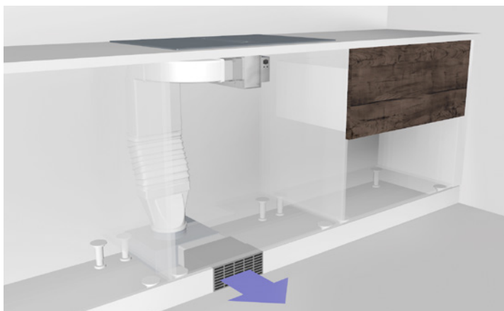
Example of installation of the H3 and H5 Filter with Surface Hoods Flow 4 & Flow 5
